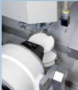
The objects are separated from the stock on the Rödgers RXD5 in a fully automatic manner.
