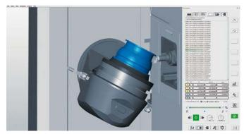
NEW: In the hyperMILL\* SIMULATION Center and in the virtual machine revolved geometries are displayed as such
