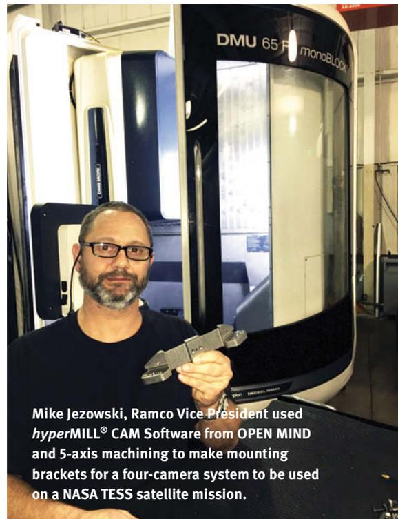
Mike Jezowski, Ramco Vice President used hyperMILL® CAM Software from OPEN MIND and 5-axis machining to make mounting brackets for a four-camera system to be used on a NASA TESS satellite mission.
