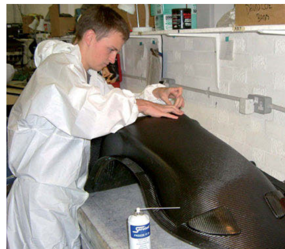
Composite Racing Seat In Production at Reverie
