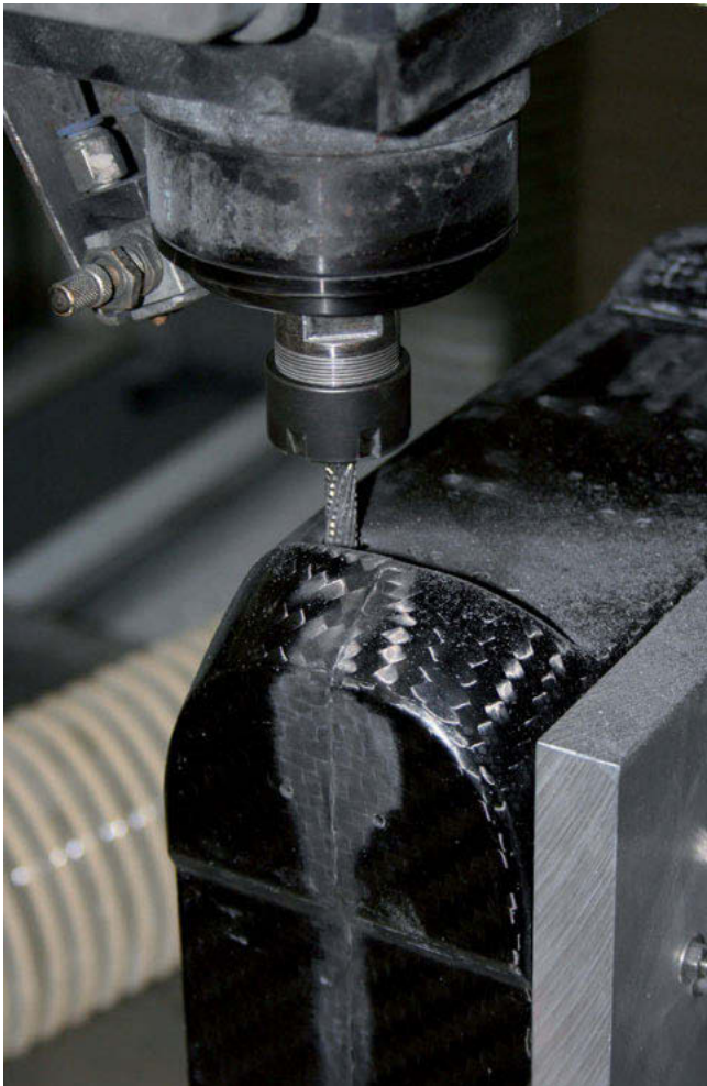
Carbon fibre electronic boxes being machined with PCD Tooling at Reverie
