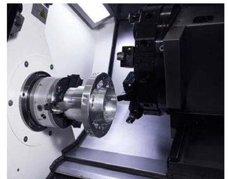
Turning with turret on a CTX alpha 500 from DMG MORI with Siemens controller
