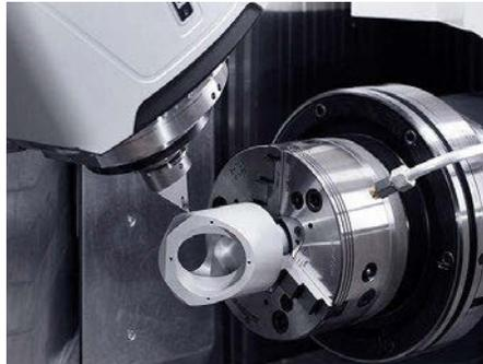
Complete machining on a DMG MORI CTX turn-mill machine
