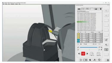
hyperMILL<sup>®</sup> VIRTUAL Machining simulates the NC code line for line, including all transition movements
