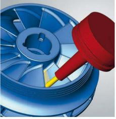
*hyper*MILL® offers safe and reliable 5-axis strategies with automatic collision avoidance when machining undercuts
