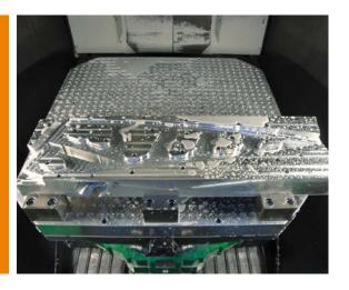
"The linking of toolpaths within the work area removes the number of rapids the machine requires during positioning. This reduces air time and keeps the tools doing what they are best at – cutting. Its the air time that costs us money. The ability of the Linking Cycles to move the tool around the work piece to the next approach position is a bonus, this move is collision checked and checked against the stock when used in production mode and this ensures the shortest possible tool path."
