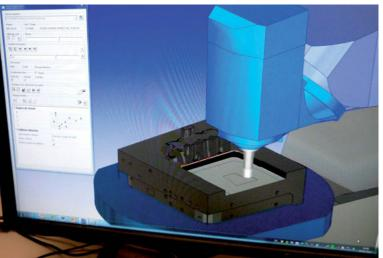
ready been created in the *hyper*MILL<sup>®</sup> software and are used daily. After these applications in 2 axes, *hyper*MILL<sup>®</sup>'s programming was quickly requested to test blank engraving capability; that is, machining complete moulds in three dimensions.
