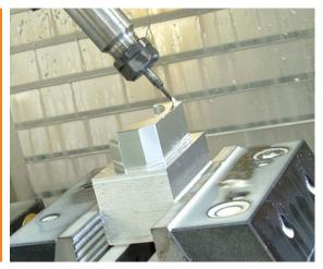
Patterns, manufactured from aluminium, tooling block or graphite, are also a common sight on the machines at CFT.
