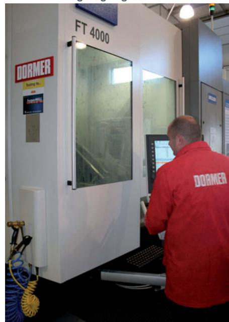
“The component has a number of pockets on each side and to demonstrate cycle time reduction with *hyperMILL*® MAXX Machining roughing strategies, one pocket was previously machined in 40 minutes. Dormer Pramet is now milling the pocket in 3 minutes.”
