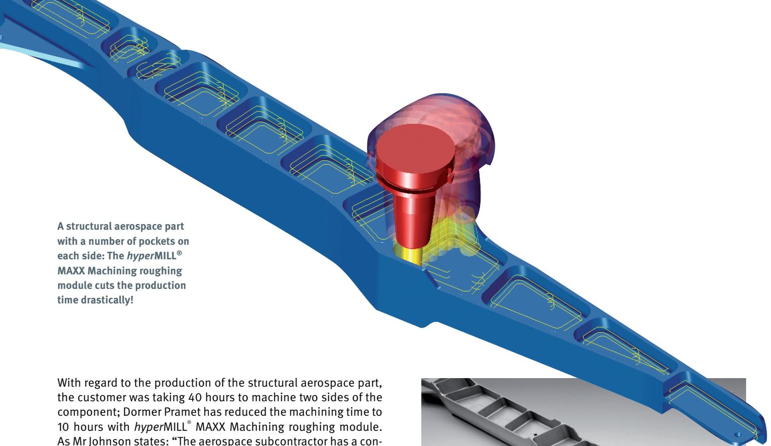
A structural aerospace part with a number of pockets on each side: The *hyperMILL*® MAXX Machining roughing module cuts the production time drastically!
